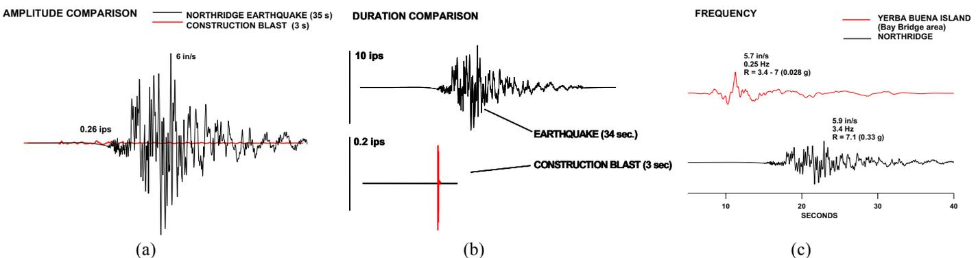
Figure (a) compares the amplitudes for a typical construction blast (0.26 in/s) in red and an earthquake (6 in/sec) in black
