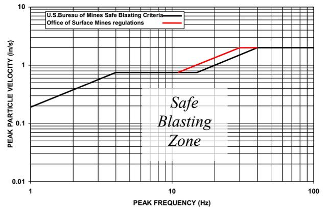
As damage is probabilistic, the USBM provided a range to *the lower limits* of peak ground motions at which three categories of damage may appear as ground velocity at the structure increases:
